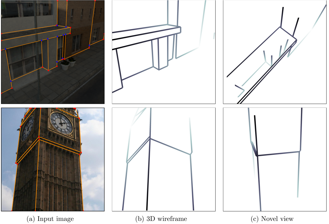
Figure 4.1: Results of our method tested on a synthetic image (top row) and a real image (bottom row). Column a shows the input images overlaid with the groundtruth wireframes, in which the red and blue dots represent the C- and T-type junctions, respectively. Column b shows the predicted 3D wireframe from our system, with grayscale visualizing depth. Column c shows alternative views of b. Note that our system recovers geometrically salient wireframes, without being affected by the textural lines, e.g., the vertical textural patterns on the Big Ben facade.
